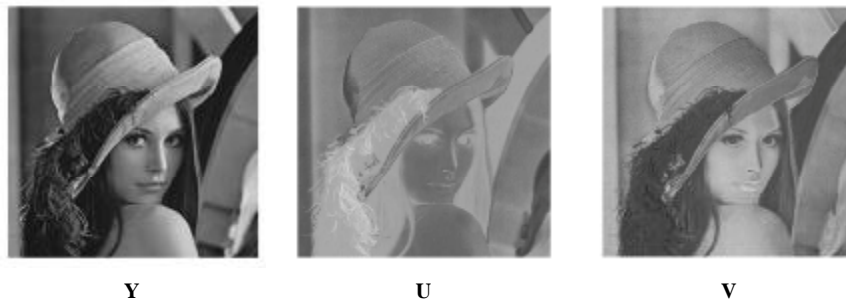
Figure 3. Converted RGB image to YUV color space
