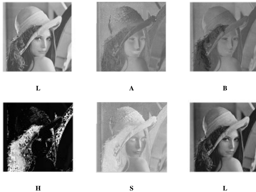
Figure 5. Representation of various color components; (a) L^*a^*b (first row) (b) HSL(second row)
