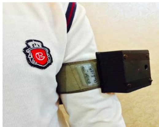
Figure 4. A customized package and the interface between the wearable device and a patient body.
